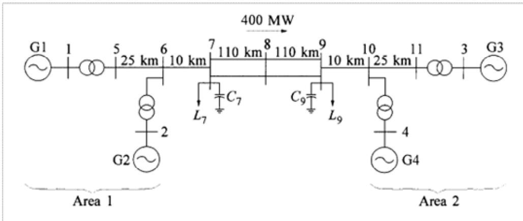
Figure 3: Test System, extracted from [12]
