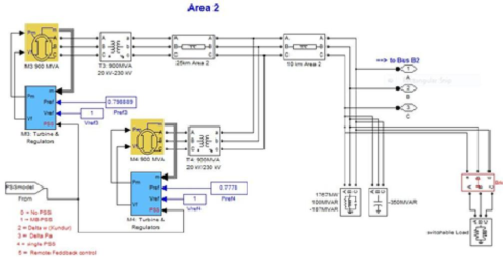
Figure 5: Area 2 subsystem with switchable loads
