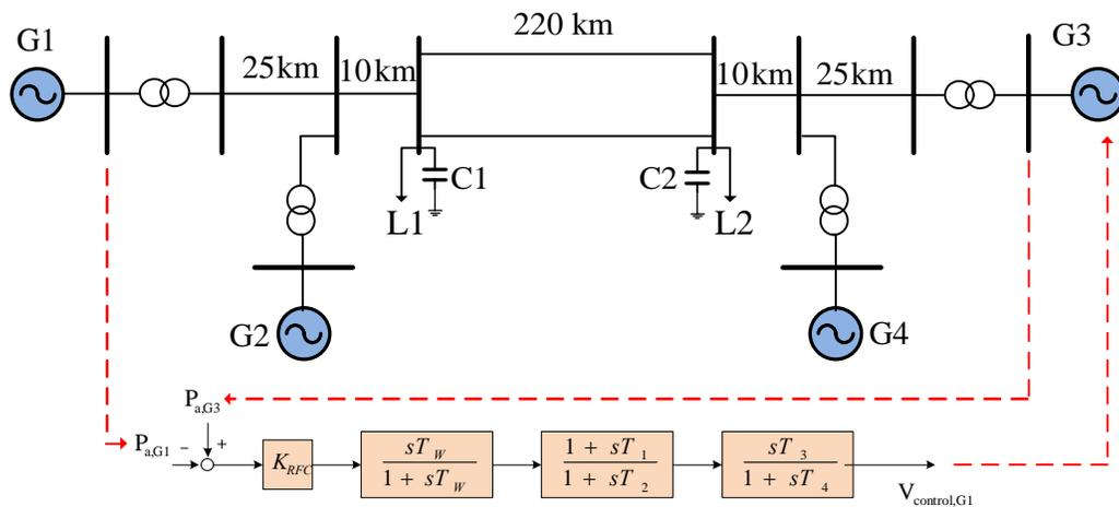
Figure 8: Test system with the remote feedback controller
