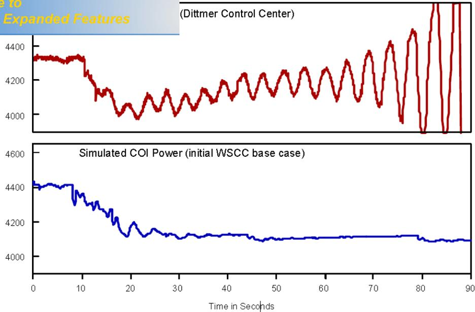
Figure 1: Comparison of observed system response during August 10, 1996 disturbance with response using models in use at that time, extracted from [7]
