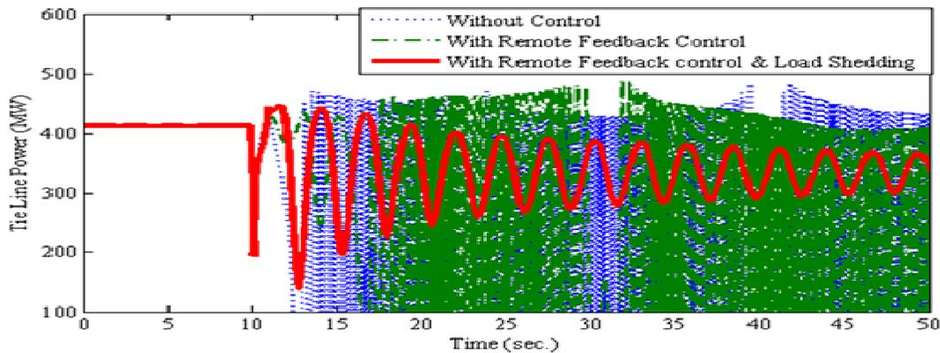
Figure 11: Line trip after 10 seconds with and without load shedding
