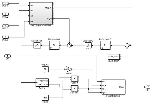
Figure 14: RFLC load controller architecture
