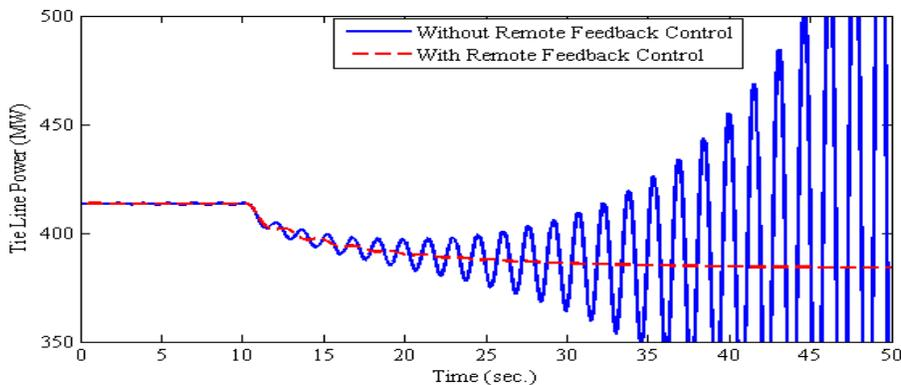
Figure 9: The tie Line power of the system without a controller vs remote feedback control at Gen 3
