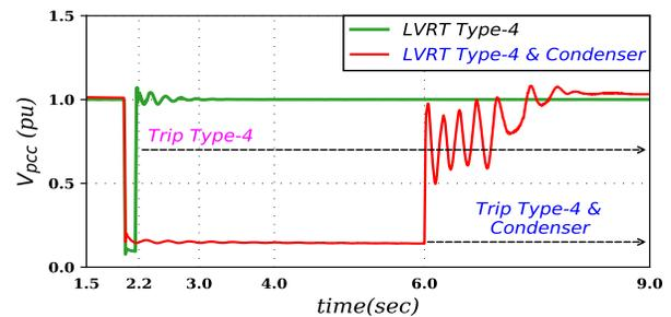
Fig. 10. LVRT capability of the system.
