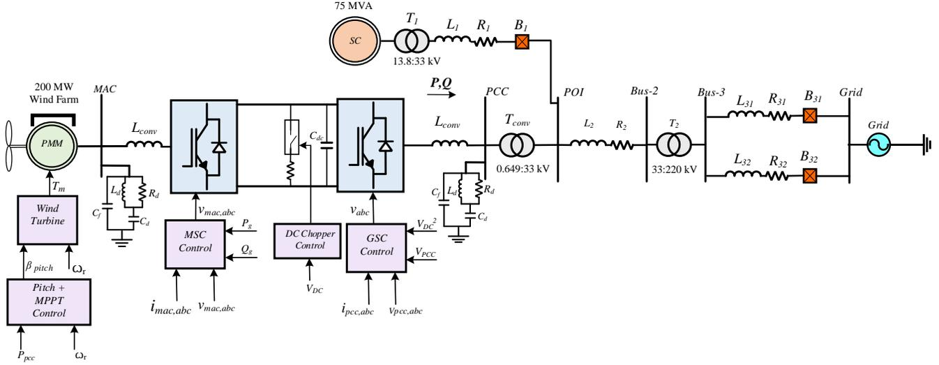
Fig. 1. PSCAD testbed: 200 MW Type-4 wind farm is connected to the grid, with 75 MVA Synchronous condenser interfaced at the 33 kV bus.
