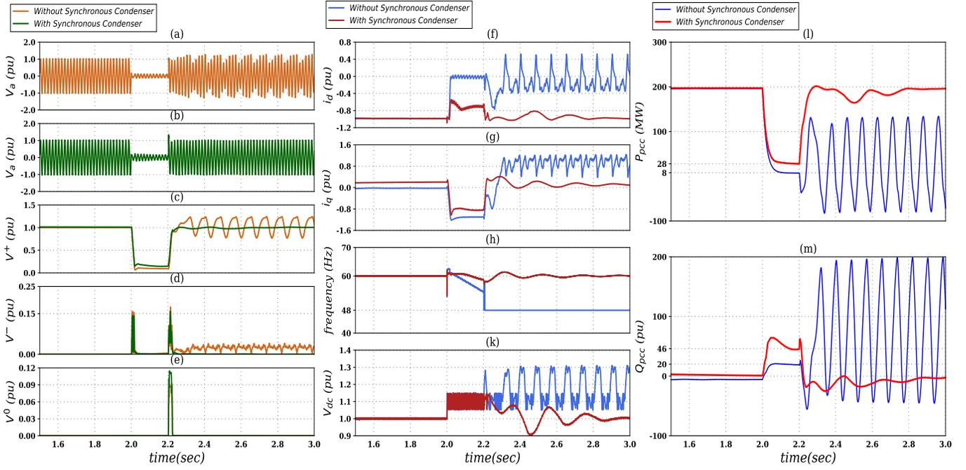
Fig. 7. Response of the system to three-phase-to-ground fault. (Fault duration = 0.2 sec)
