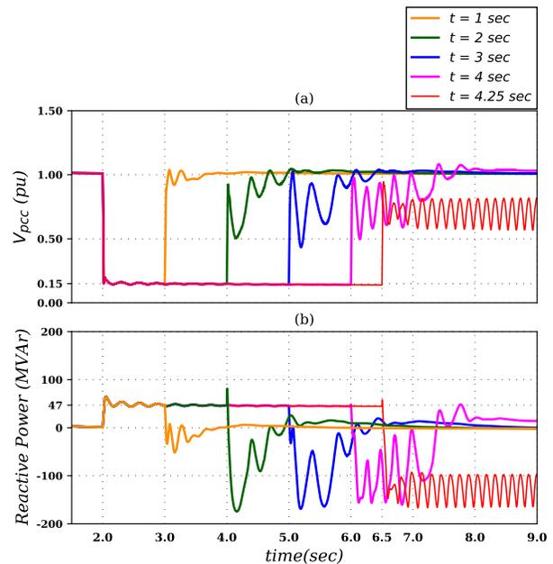
Fig. 9. LVRT capability of Type-4 with Synchronous condenser connected.
