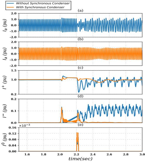
Fig. 8. Current injected by the type-4 wind during a three-phase-to-ground fault
