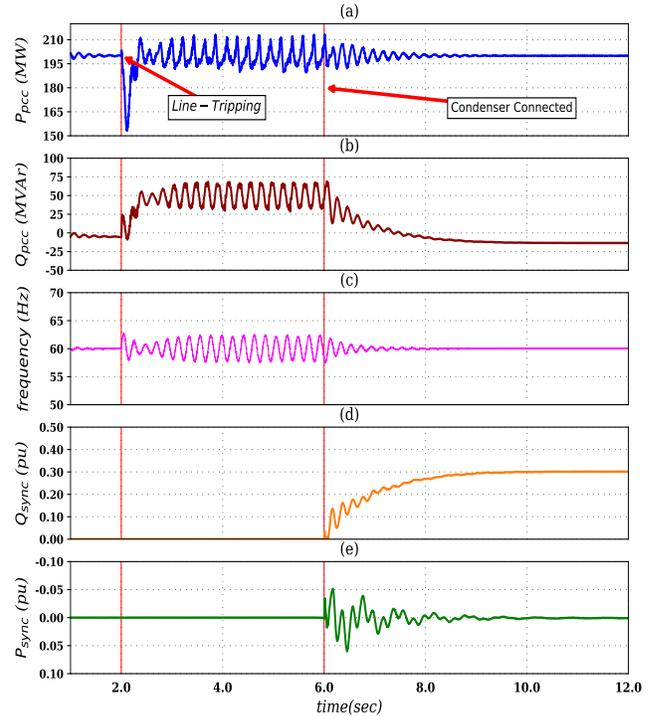
Fig. 3. Transient responses of the system when a fault occurs at  $t = 2$  s and at  $t = 6$  s the synchronous condenser is connected.
