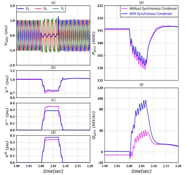
Fig. 5. Response to a single-phase-to-ground fault with and without the synchronous condenser.
