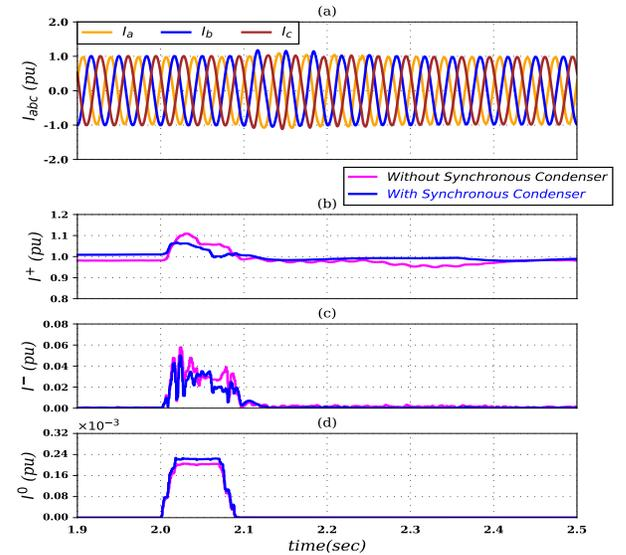
Fig. 6. Current injected by the type-4 wind during a single-phase-to-ground fault
