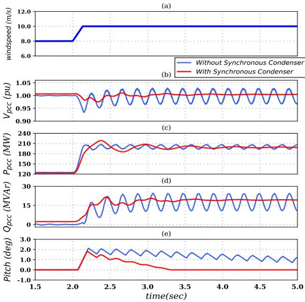
Fig. 4. Response of type-4 to increase in wind speed (8 to 10 m/s) in a weak grid scenario and when the synchronous condenser is connected in parallel.
