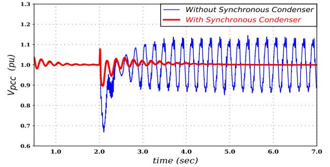
Fig. 2. Type-4 wind system performance with and without Synchronous Condenser in a weak grid scenario
