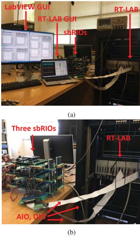
Fig. 5: (5a) The photo of CHIL testbed built in our lab. (5b) zoom-in photo to show the detailed connections of RT-LAB and sbRIOs.
