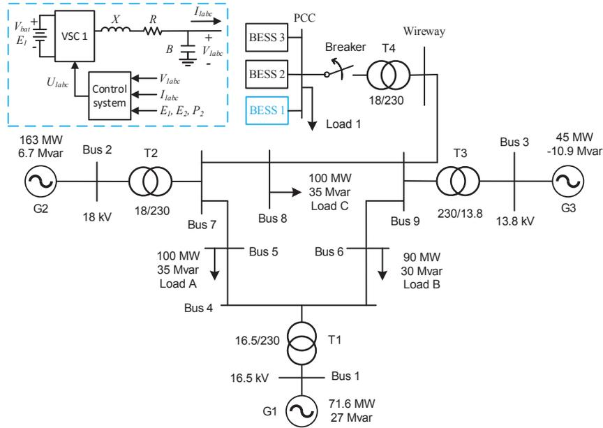
Fig. 3: The microgrid including three energy storage systems is integrated to IEEE-9 Bus system.
