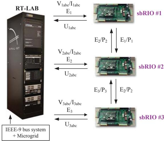
Fig. 4: The overview of CHIL testbed.
