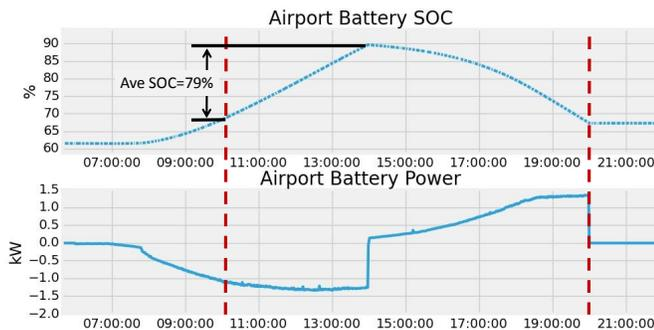
Fig. 10: Airport battery SOC cycle sample with small SOC deviation.
