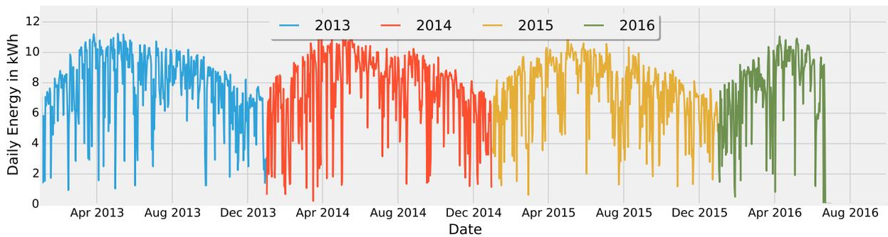
Fig. 7: 2013-2016 airport PV daily energy in kWh.
