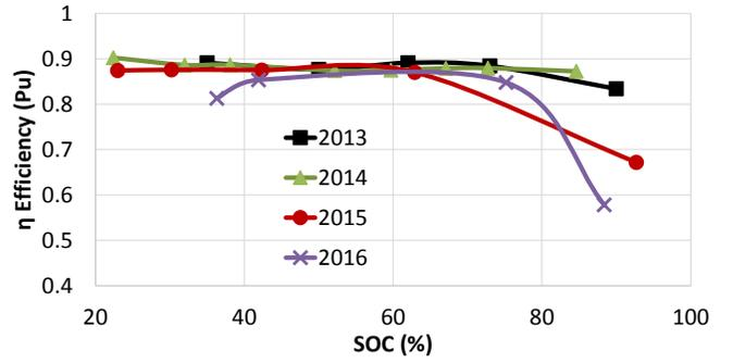
Fig. 11: Airport battery efficiency at different SOC levels.
