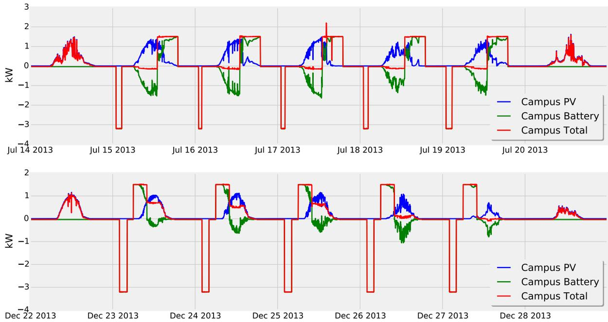
Fig. 5: Campus PV/Battery system summer (upper one) and winter (lower one) operations.
