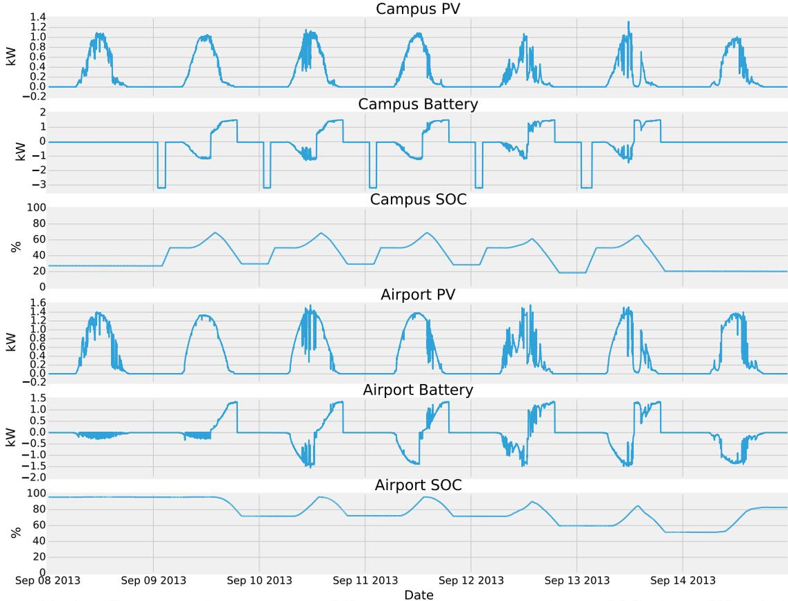
Fig. 3: A week's data. From top to bottom: campus PV, campus battery, campus battery SOC, airport PV, and airport battery, airport battery SOC. Note for batteries, reference power direction is assumed to be discharging.
