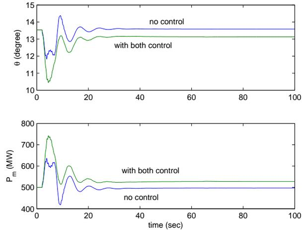
Fig. 13. Comparison of the dynamic responses of the pitch angle and wind power  $P_m$ .
