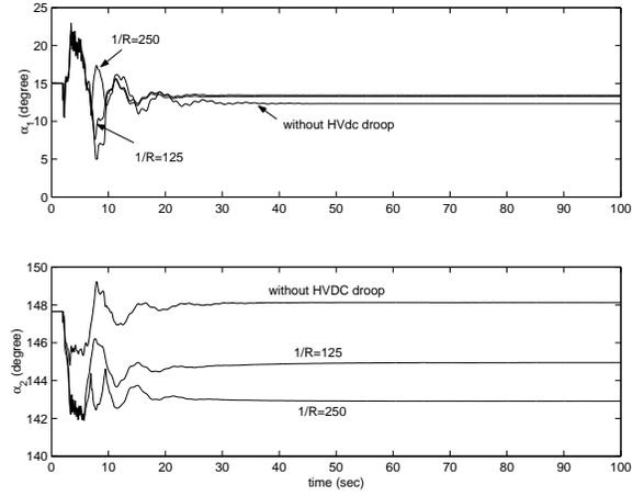
Fig. 11. HVDC converter firing angles.
