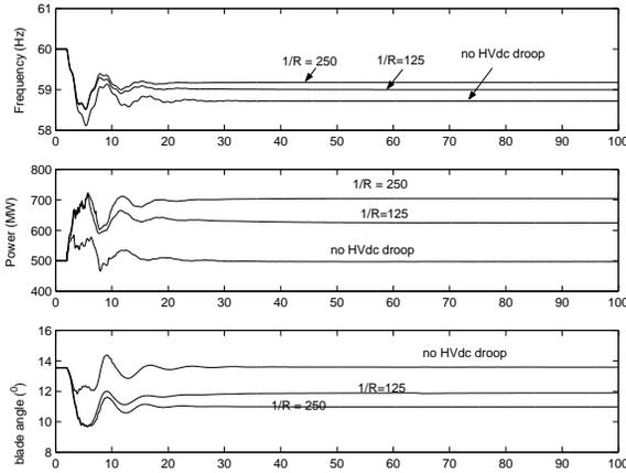
Fig. 10. Wind generator power output and system frequency.
