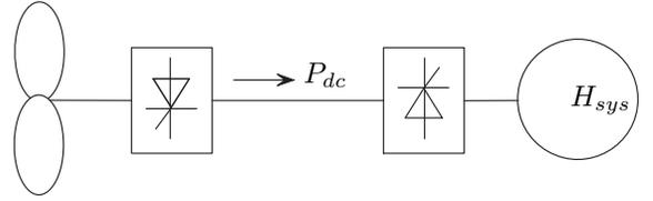
Fig. 3. A wind farm with HVDC delivery connected to a system with aggregated inertia  $H_{sys}$ .
