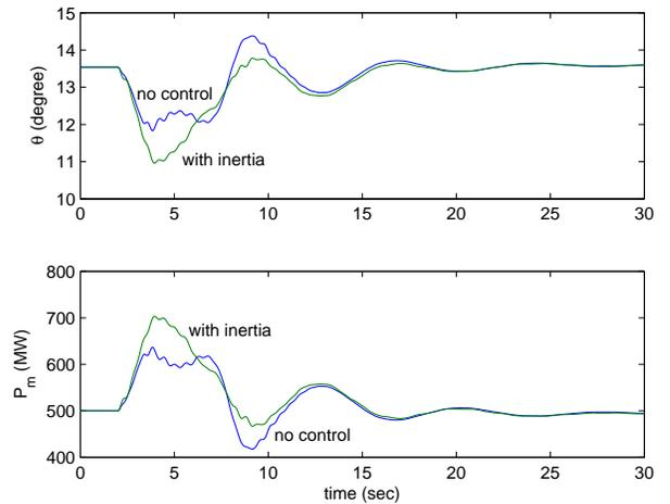
Fig. 9. Comparison of the dynamic responses of the pitch angle and wind power  $P_m$ .
