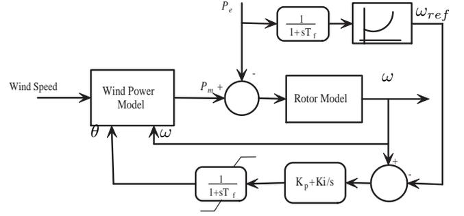
Fig. 5. Block diagram of a wind turbine.
