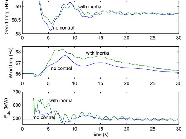
Fig. 8. Comparison of the dynamic responses of the system frequency, wind speed and  $P_{dc}$ .
