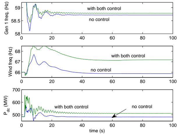
Fig. 12. Dynamic responses of the frequency of Gen 1, Wind Gen and  $P_{dc}$ . a) no control; b) with both inertia enhancement  $K = 100$  MW/Hz and frequency droop  $R = 50$  MW/Hz.
