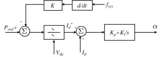
Fig. 2. Control loop for HVDC rectifier with enhanced inertia loop.
