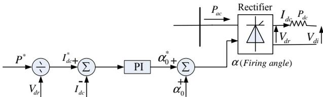
Fig. 1. Constant power control diagram.
