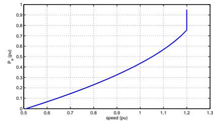
Fig. 6. Reference speed versus electric power output from a wind generator.
